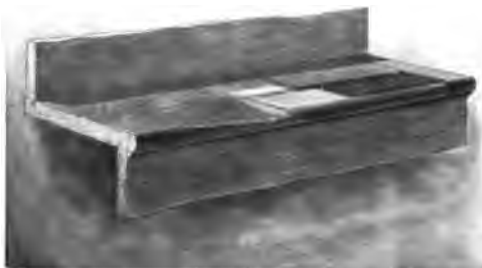
Fig. 2. Method of Repairing Worn Tread.
